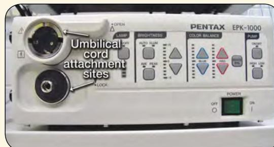
Figure 6. Pentax light source unit
