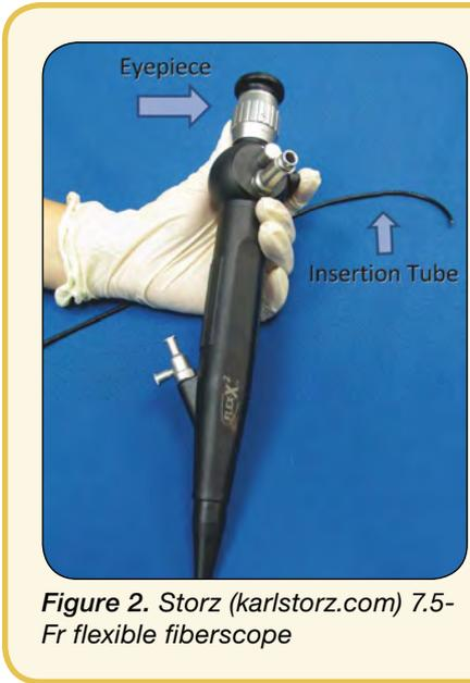
**Figure 2.** Storz (karlstorz.com) 7.5-Fr flexible fiberscope
