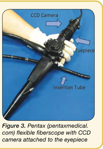
**Figure 3.** Pentax (pentaxmedical.com) flexible fiberscope with CCD camera attached to the eyepiece
