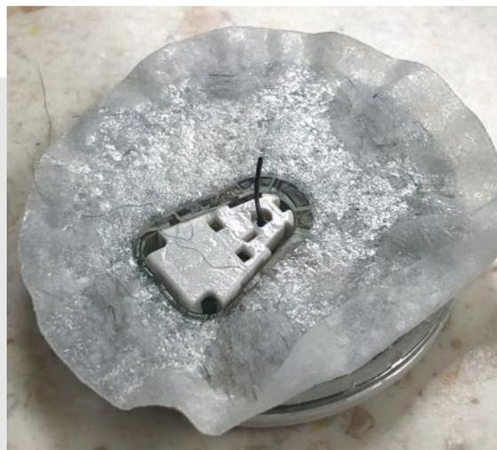
**FIGURE 1.** The adhesive side of a CGM sensor, after removal from a patient, showing the flexible polyurethane probe that stays in the interstitial space.
