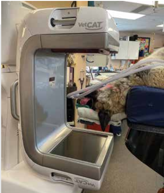
FIGURE 1. Working area of a cone beam computed tomography system. The x-ray generator and a flat collection plate are on opposite sides of the patient. The machine makes a single rotation around the patient to collect the data.
