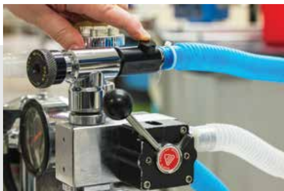
FIGURE 1. Pop-off button placed between the pop-off valve and the scavenging system. When pressed, the button closes the system, allowing a positive-pressure breath to be administered by the anesthetist. When the button is no longer pressed, it automatically opens; thus, the system is never closed for longer than it takes to give a breath.
