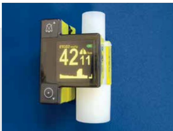
FIGURE 2. A mainstream capnograph, the EMMA, displays the numerical value and capnography waveform.
